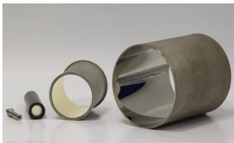
Figure 4 (left) shows different structures of these replicated optics which can be used from hard x-rays (8 keV leftmost in the picture) to several 100 eV (rightmost in the picture).
